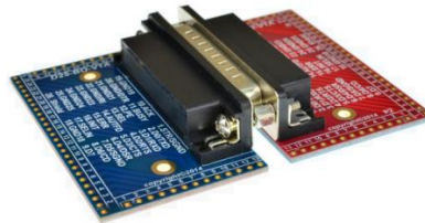
Figure 5: Solid Male to Female connection with the 4-40UNC diameter 8.3mm long screws
